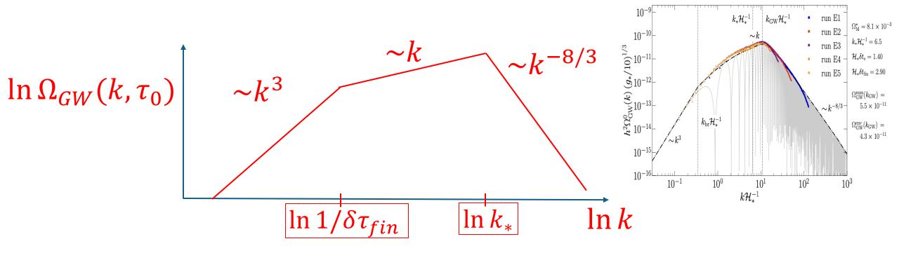
GW spectrum from sound waves (in the sound shell model) can be understood from the properties of the self-similar profiles and of the bubble nucleation history
